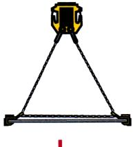
Chain ropes equipped in metal sheets lifters
